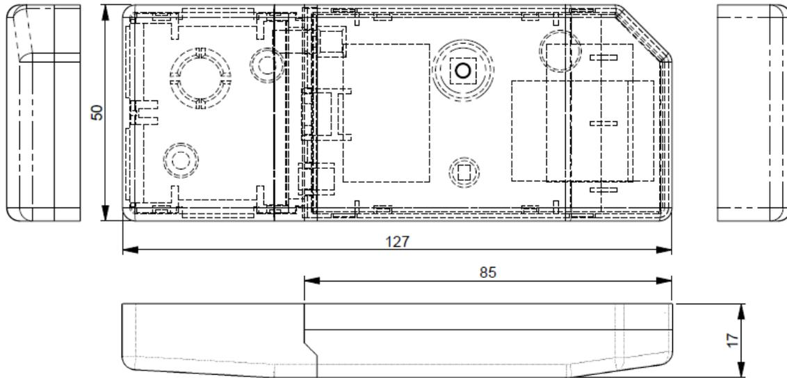
**Figure 2.1** Device dimensions in mm and back view
