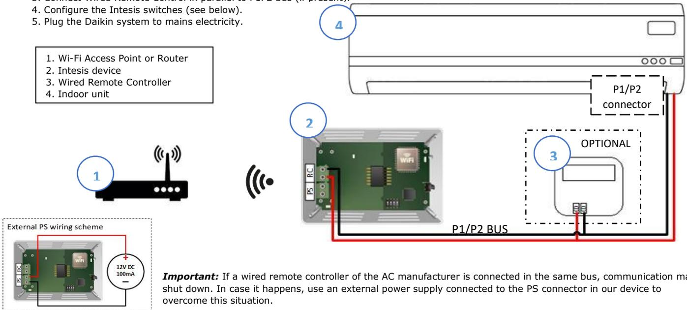
**Important:** If a wired remote controller of the AC manufacturer is connected in the same bus, 12V communication may shut down. In case it happens, use an external power supply connected to the PS connector in our device to overcome this situation.
