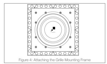
Install the grille on to the grille mounting frame. The powerful Neodymium magnets will attract the grille very quickly. Care should be taken to align the grille correctly before placing it close to the grille mounting frame (see Figure 5).
