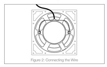
3. Attach the woofer driver to the enclosure using the twelve Phillips head screws.
