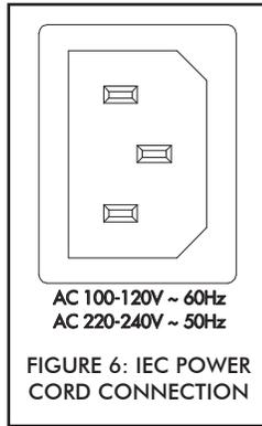
FIGURE 6: IEC POWER CORD CONNECTION
