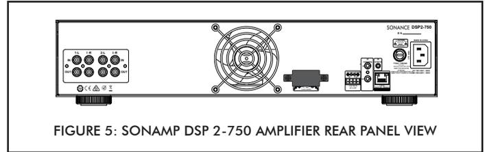
FIGURE 5: SONAMP DSP 2-750 AMPLIFIER REAR PANEL VIEW
