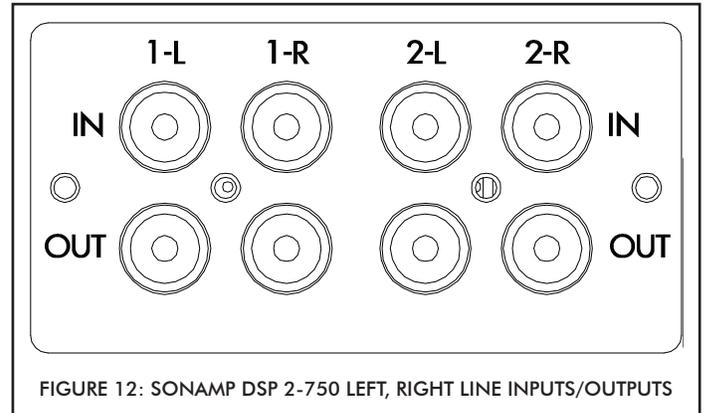
FIGURE 12: SONAMP DSP 2-750 LEFT, RIGHT LINE INPUTS/OUTPUTS
