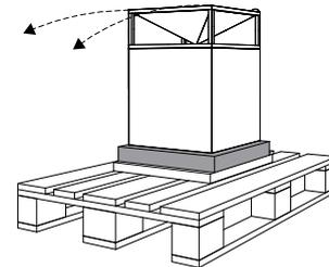
Remove the foam packing protecting the module inside the box. Holding the Cube from the metal base gently turn the module, tilting it into position.
