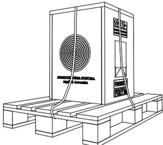
Due to its size and weight, the Cube is shipped in a wooden box, secured to a pallet with strapping to allow its handling and movement into position with a forklift.
