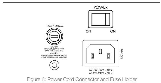
Figure 3: Power Cord Connector and Fuse Holder
