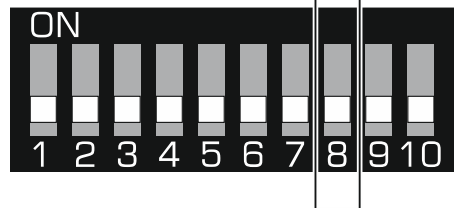
Fig. 3. Switch defining which antenna will be used for transmitting.
